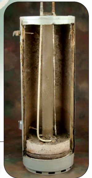
Example of mineral buildup in an unprotected water heater.
